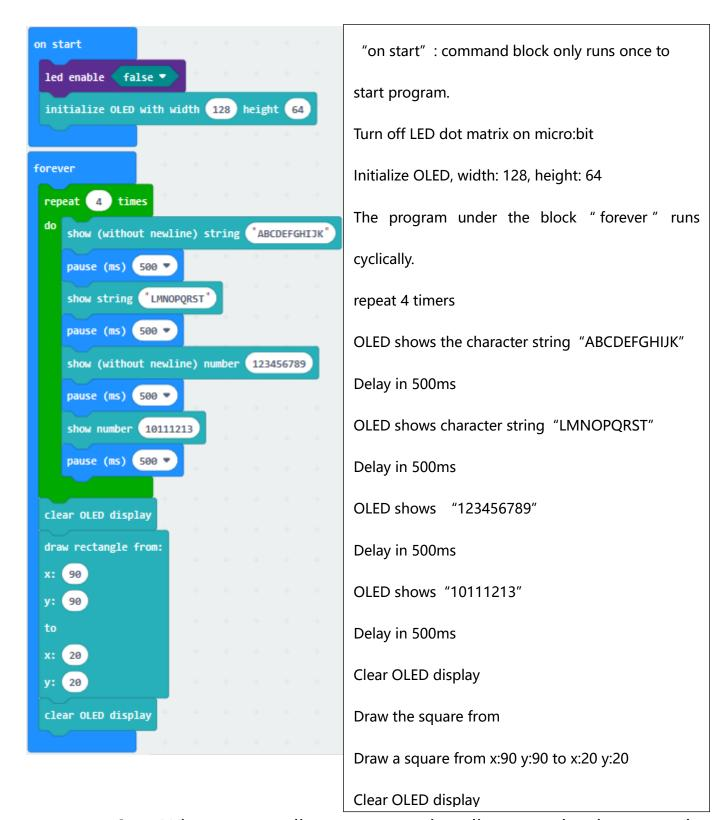
**Test Results:** Wire up according to connection diagram. plug in external power and upload code to micro:bit, the corresponding character and patterns are displayed on OLED.
